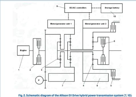
Fig. 2. Schematic diagram of the Allison EV Drive hybrid power transmission system [7, 10]: 1 - IC engine; 2 - clutch; 3 - dual-ratio planetary gearset; 4 - planetary gearset;
