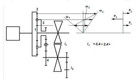
Option III: CVT connected with the sun gear and engine connected with the ring gear
