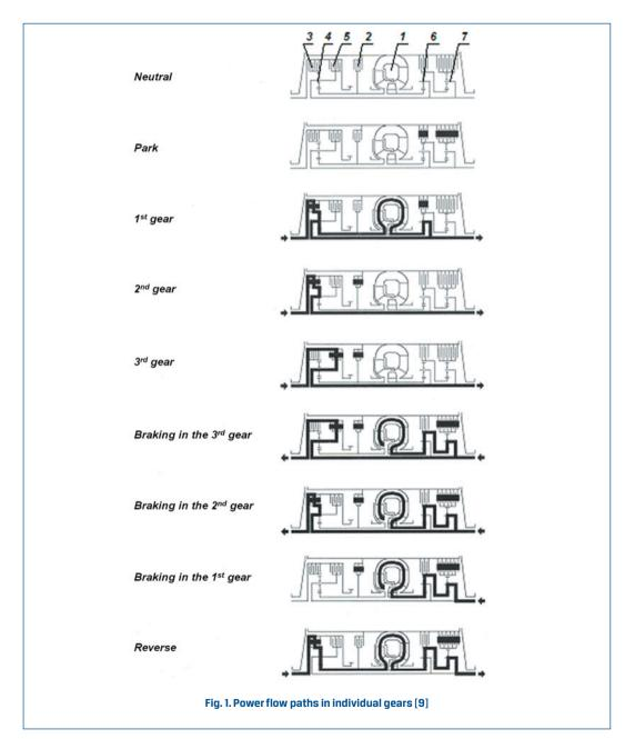
The reversing is done with the use of splitting gearset 4, hydrokinetic torque converter 1, and reversing planetary gearset 7. The achievable driving force is equal to that developed in the 1st gear and the maximum driving speed is equal to 0.1 V<sub>max</sub> (0.1 of the maximum speed of the vehicle when driven forwards).
