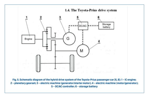
In the hybrid drive system of the Toyota-Prius passenger car, the vehicle may be driven either by its electric motor only (at low acceleration or when moving with a constant speed) or both by its electric motor and IC engine (at higher loads), see Fig. 5 [6, 8]. The IC engine is
