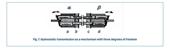
The  $\alpha$  and  $\beta$  members (subassemblies) of the hydrostatic transmission may operate interchangeably as a pump and motor, in both directions of the power flow.
