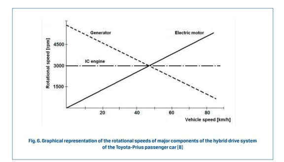
The electric machines used are high-efficiency brushless permanent magnet synchronous machines of 50 kW power capacity at 500 V rated voltage and of 400 Nm maximum torque, which is practically constant over the 0 to 1 540 rpm speed range. The total power available from both the power sources reaches 85 kW at vehicle speeds exceeding 80 km/h.
